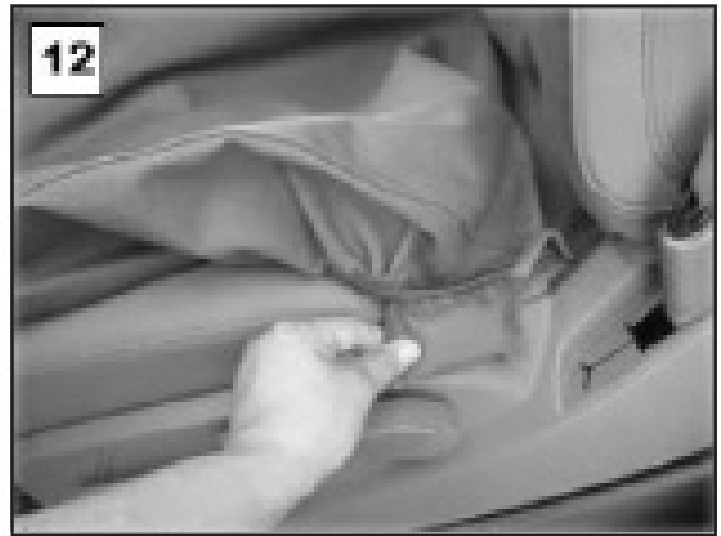
Attach pillow to the side of the seat frame Tuck pillow behind sideshield
