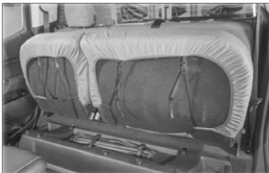
Push Cover between the seat back and bottom to secure cover
