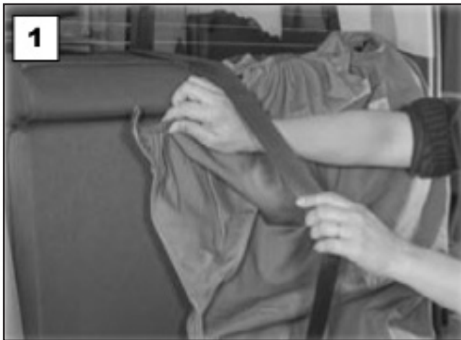
1 Place Cover under and around seatbelt
