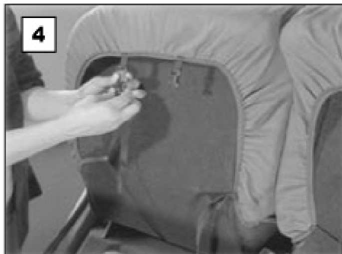
Push Cover between the seat back and bottom to secure cover
