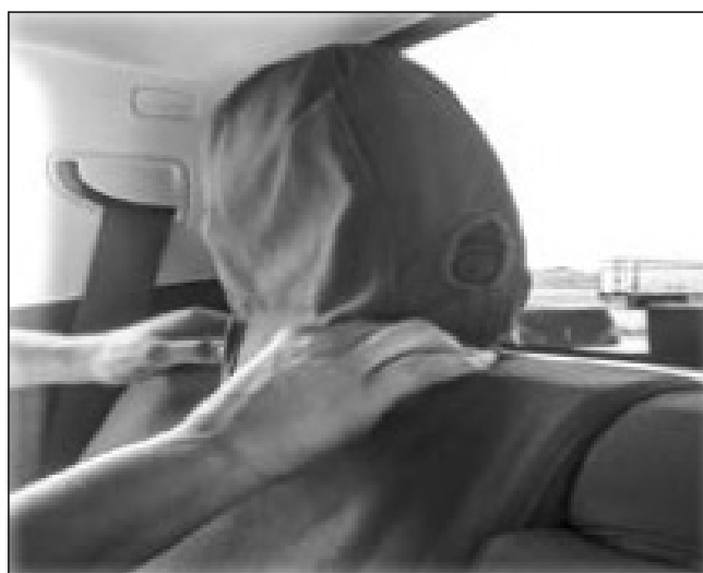
Align the cover on the headrest opening
