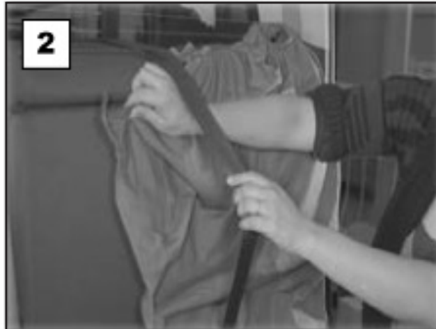
2 Place Cover under and around seatbelt
