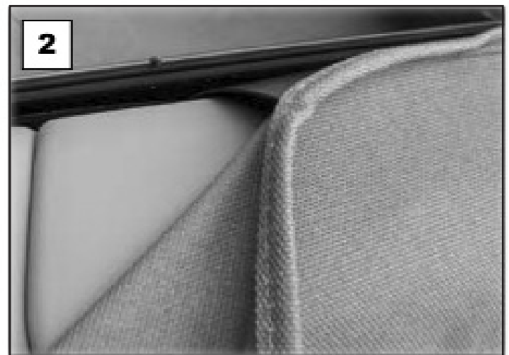
2 Slide plastic tabs in between window and seal
