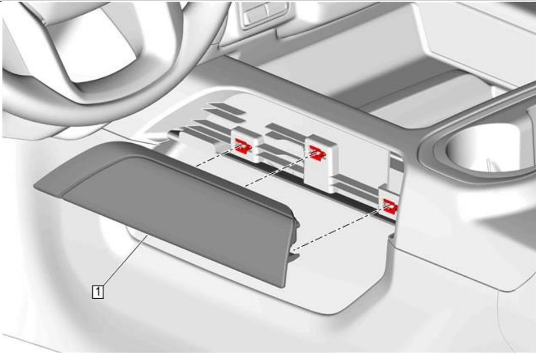
3. Using a flat-bladed plastic trim tool, release the retainer clips and remove the front floor console applique (1), if equipped from the front floor console. Repeat for opposite side.
