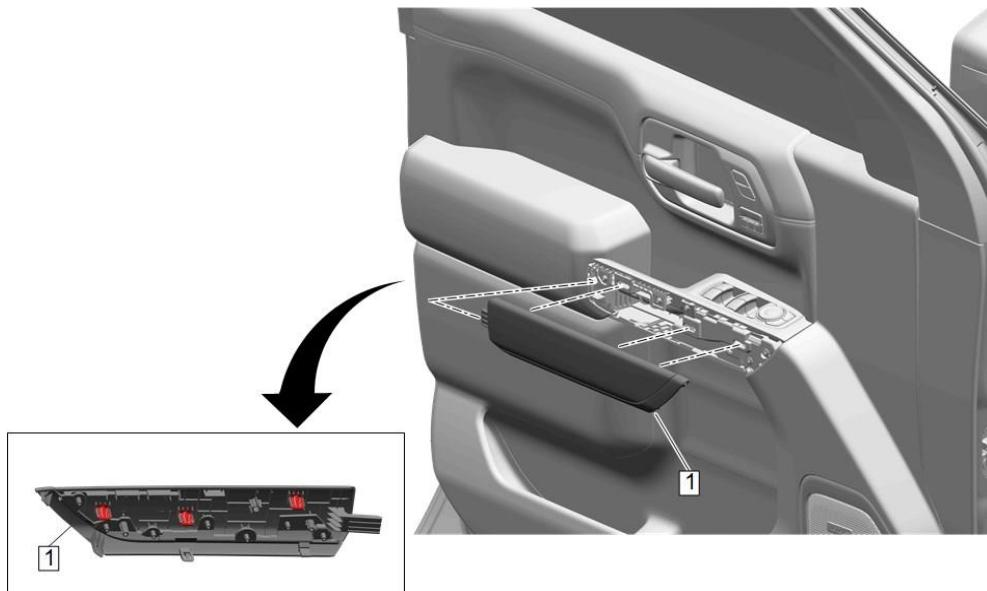
1. Using a flat-bladed plastic trim tool grasp and pull the front door armrest trim cover (1) from the bottom to unclip, then slide forward to unhook it from the front door trim panel. Repeat for opposite side.
