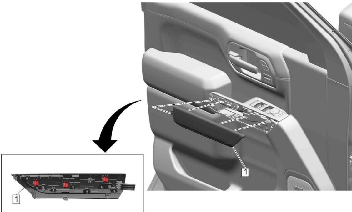
3. Position the new front side door armrest trim cover (1) outward and rearward to engage the integral hook while rotating to engage the retaining clips. Repeat for opposite side.
