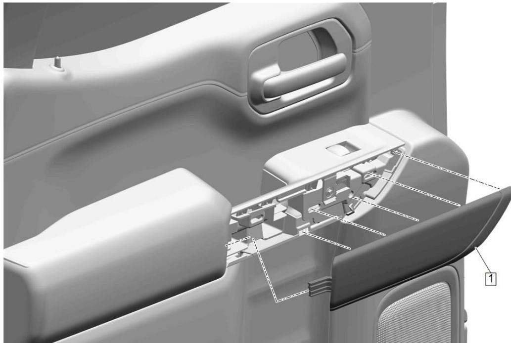
2. Start at the top front and work rearward with a flat-bladed plastic trim tool to unclip from the rear door trim panel while rotating the rear side door armrest trim cover (1) inward and forward to disengage the integral hook. Repeat for opposite side.
