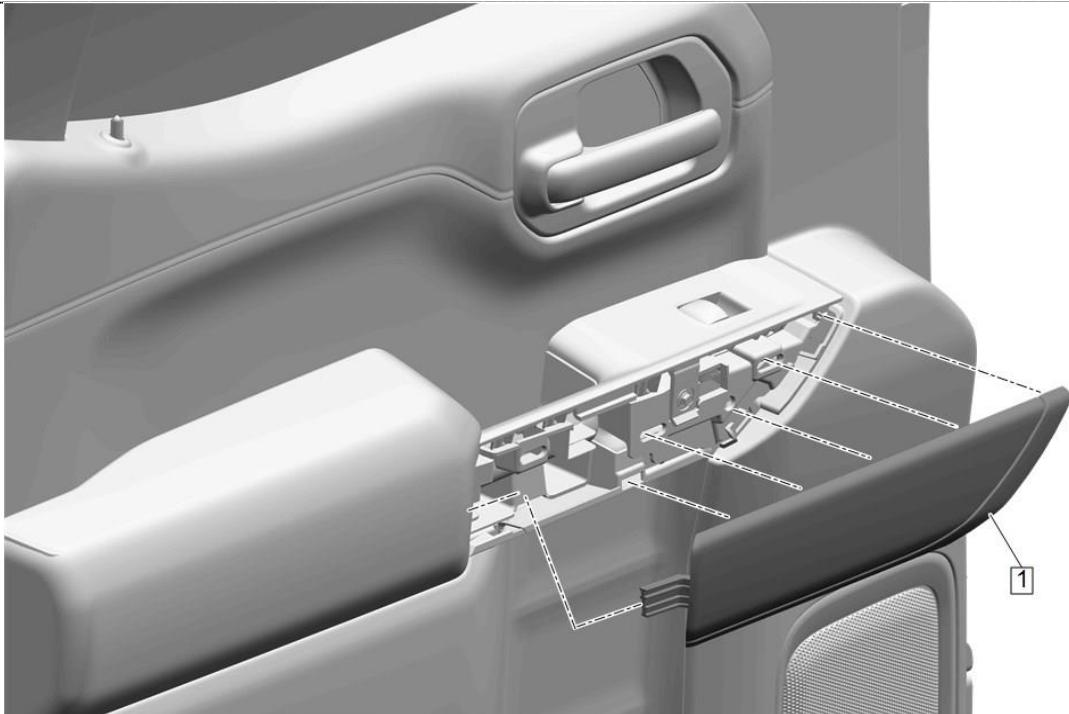
2. Position the new rear side door armrest trim cover (1) outward and rearward to engage the integral hook while rotating to engage the retaining clips. Repeat for opposite side.
