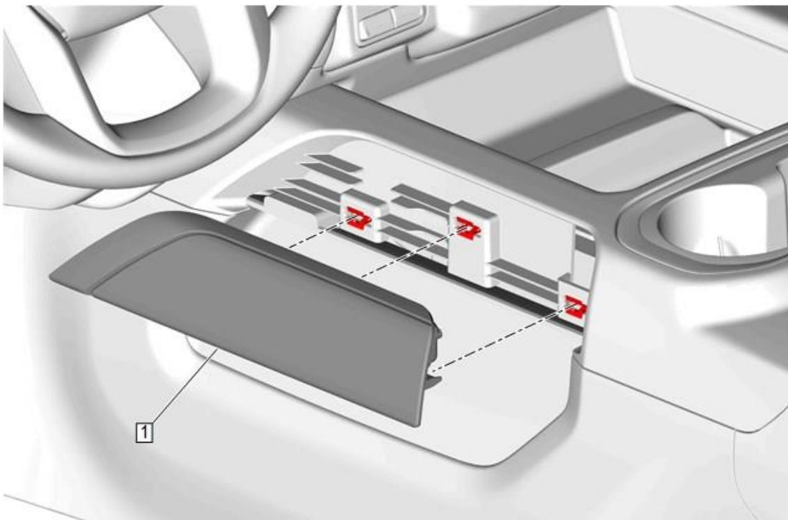
1. Position the new front floor console applique (1), if equipped to the front floor console making sure to engage the retaining clips. Repeat for opposite side.
